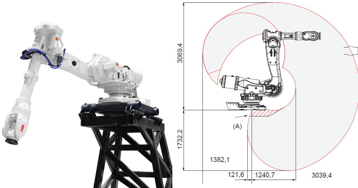
Figure 2 - The ABB 6650s and the arms span can be seen above
