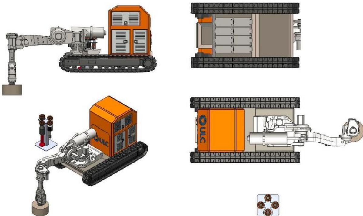
*Figure 3 - Compact Design of the Mobile Platform – (Top Left) Side View (Top Right) Bottom view of the system, (Bottom Left) Isometric View of the system with a portable tool changing rack at the operation site (Bottom Right) Top view of the system with a portable tool changing rack*
