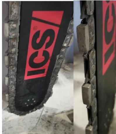
*Figure 3 - Chainsaw teeth showing diamond grit segment*
