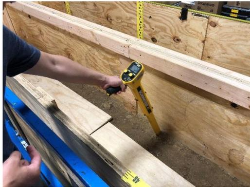
*Figure 12 – Magnetometer Soil Box Test*
