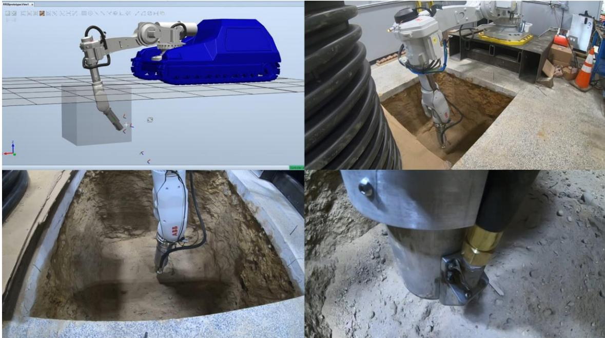
Figure 7 - Excavator head mounted at the end of the robotic arm
