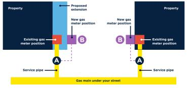
Your service pipe will normally run underground from your meter to the gas main in your street To keep you safe, you are unable to build over existing gas pipes
