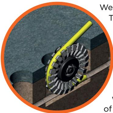
We are currently developing element two with our project partner, TRACTO-TECHNIK, who has modelled, manufactured and begun testing a new mains insertion wheel and PE pushing/pulling machine. The insertion wheel is designed to fit within three interlinked core holes, but it can also be used within a standard excavation.
