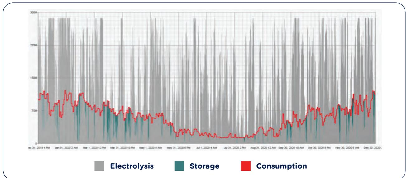
**FIGURE 28: Operation of an electrolyser with dedicated RES generation to fuel a hydrogen grid and mobility end uses combined**
