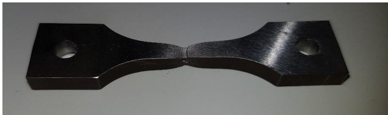
Figure 6: Typical example of a failed X42 steel tensile specimen.
