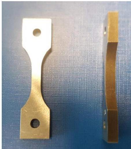
Figure 1: X42 carbon steel tensile specimens.
