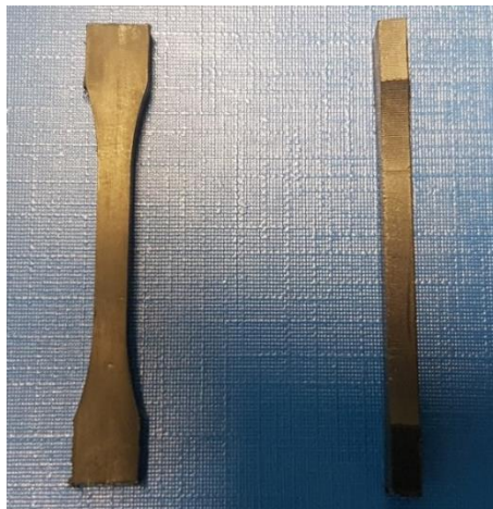
Figure 2: PE80 tensile specimens.
