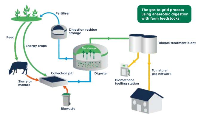
The most efficient use for this biogas is to clean it up and inject it into the gas network. Biomethane is regarded as a low-cost and scalable form of renewable and low carbon heat, which can help towards the country's energy goals.
