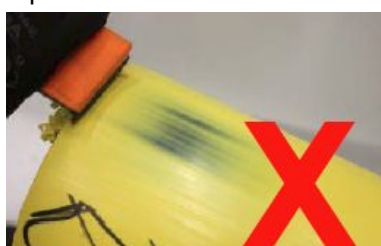
Figure D23 – DO NOT Over Scrape
