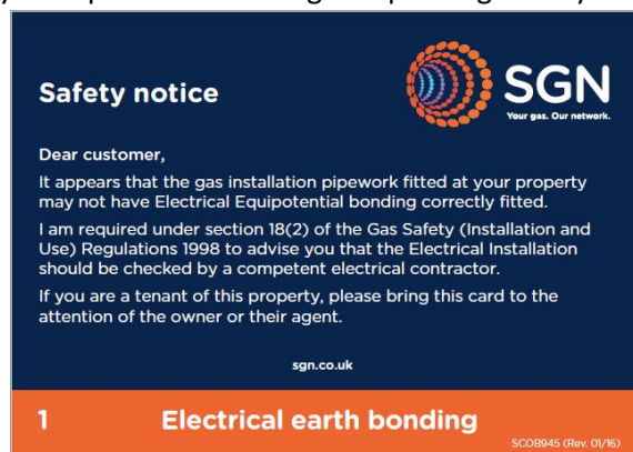
Figure O2 – Earth bonding warning notice
