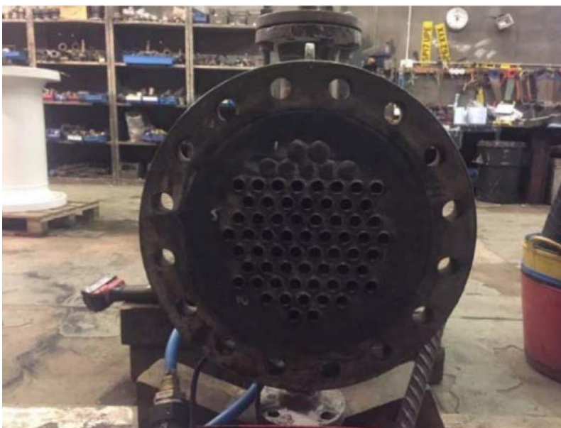
Figure 6: The end plate of a shell and tube heat exchanger
