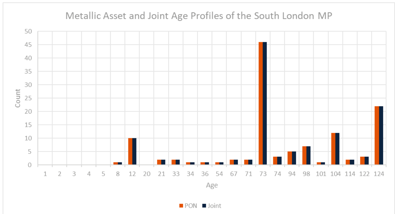
Figure 3: Age profile of the Metallic assets on the South London MP network
