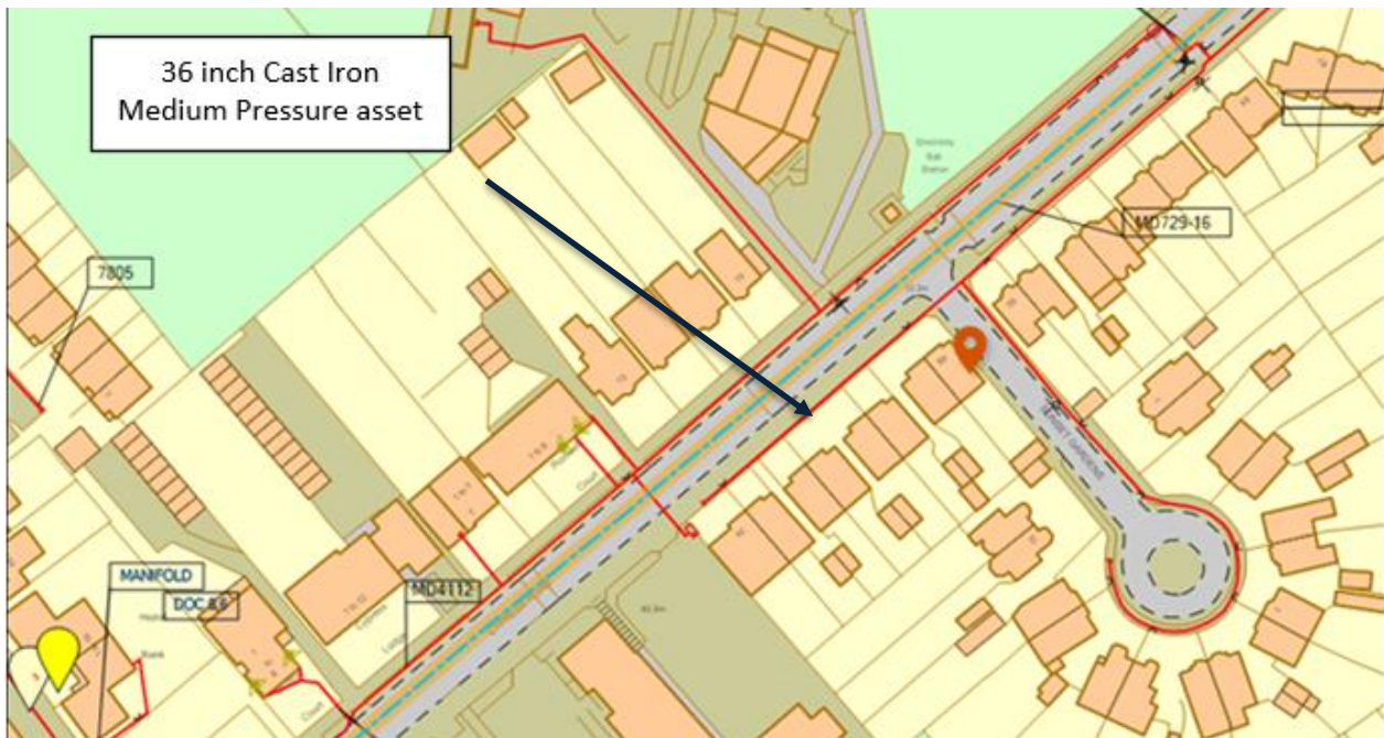
Figure 9: Asset #115789967 a 36-inch Medium Pressure mains which runs through Cypress Road
